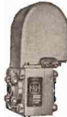
Differential Pressure (d/p) Cell
